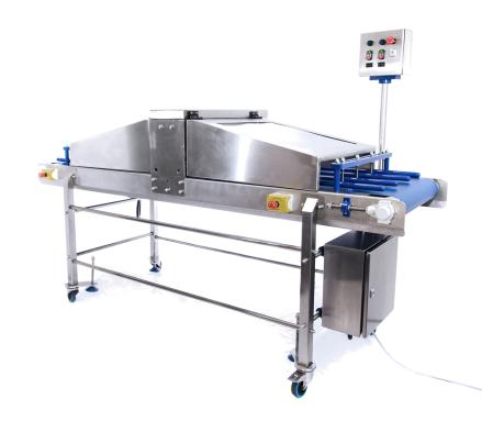
The maximum overall height of product that can be handled is 150mm. Depending on the diameter or width of product to be sliced, extra lanes can be incorporated on the 600mm wide conveyor greatly enhancing production throughput.
